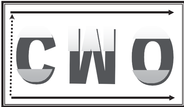
Fig. 1 Normal scan ( pin 17, reLR = Low or NC, pin 18, reUD = Low or NC )
