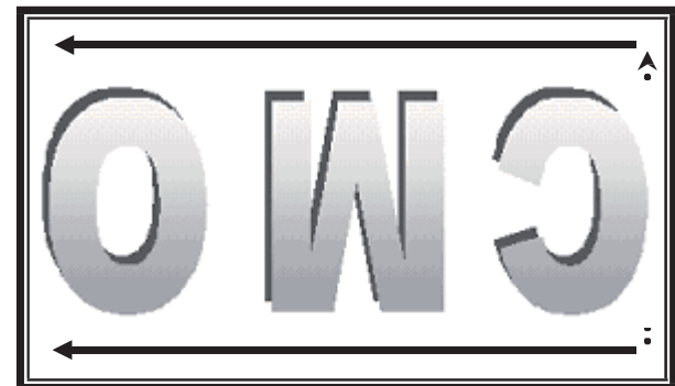
Fig. 1 Normal scan ( pin 17, reLR = Low or NC, pin 18, reUD = Low or NC )
